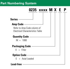
Notes: \* 0.1A-6A have 0.65±0.05 diameter lead. 7A have 0.8±0.05 diameter lead.
